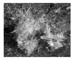
FIGURE 26. Mycelium of *Penicillium* around crystals of ammonium dihydrogen phosphate. The fire retardant salt had been added to the plywood used for the roof deck. The picture is about 1.5 mm across.
