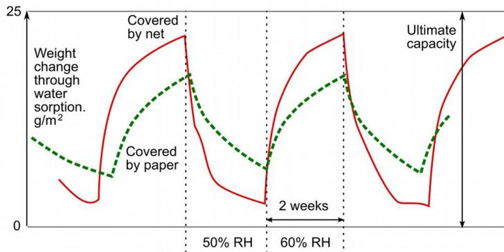
FIG 4. The effect of covering unfired perforated brick with a single layer of filter paper. The response curves to a four week square wave RH cycle are plotted superimposed. The top and bottom boundary lines indicate the ultimate buffer capacity derived from the static sorption measurement. The net had mesh openings 1.2 mm square, the paper was Whatman no.1, 88 g/m<sup>2</sup>.
