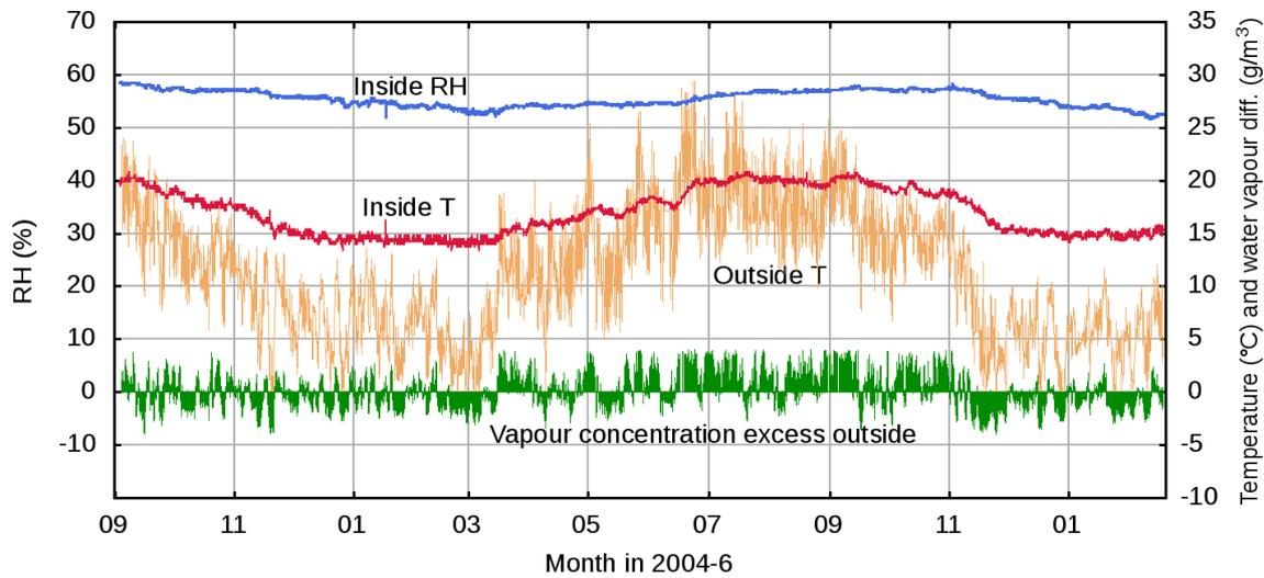
FIG 1. The annual cycle of temperature and relative humidity in the Suffolk Record Office. The lowest trace indicates the difference between the concentration of water vapour inside and outside. During the winter the inside RH is driven down by air exchange; during the summer the outside air has a higher water vapour concentration, as shown by the lowest trace being mostly above the zero line, but buffering by the archived documents slows the rise of indoor RH.
