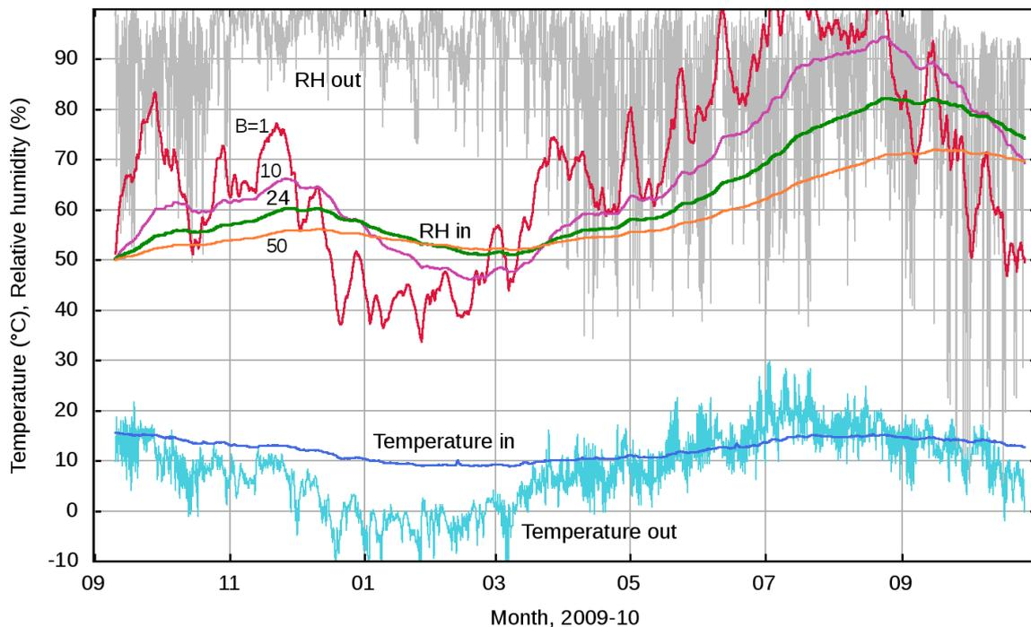
FIG 5. Simulated buffering of the RH in a museum store by lining the walls with unfired brick (trace 24). The interior RH starts arbitrarily at 50%. The trace marked  $B=1$  shows the course of the RH in a completely water-inert building with an air change rate of  $0.03 \text{ h}^{-1}$ .
