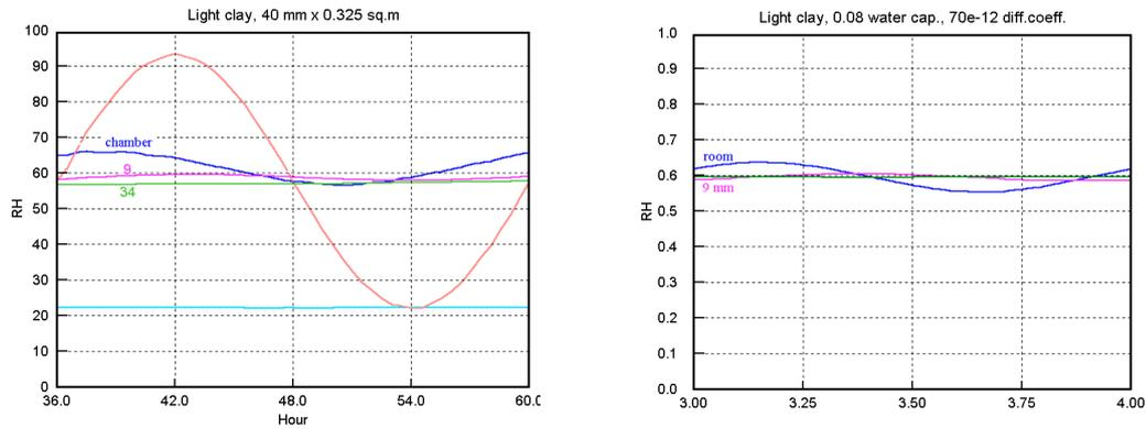
Figure 5.6 A: On the left is the measured performance of the test wall under a daily flux cycle. B: On the right is the modelled performance, which shows a slightly too good stabilisation of the climate.
