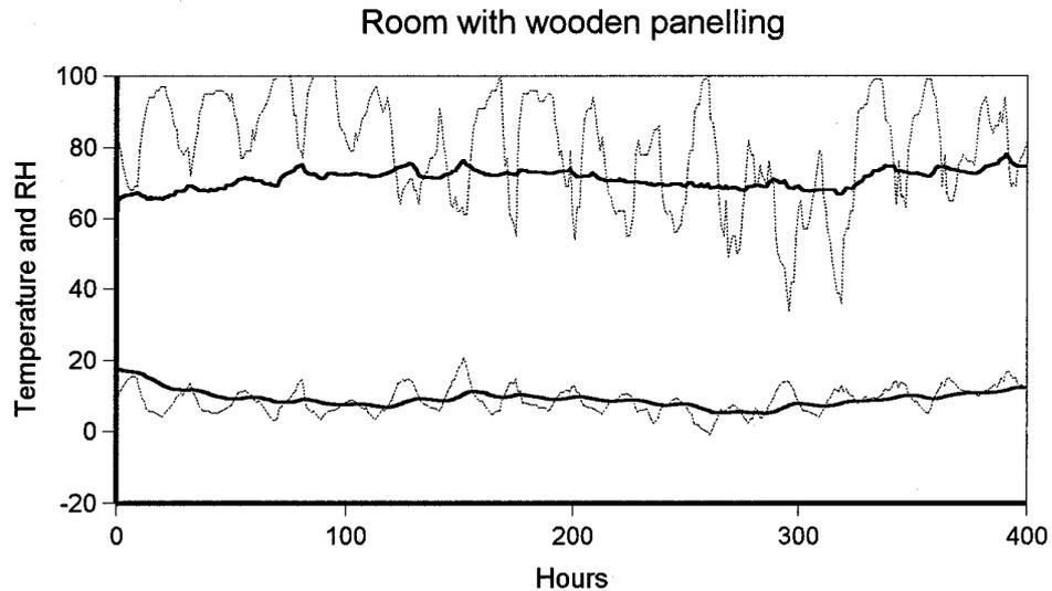
*Figure 5.12 The climate over 12 days inside a room 10 x 10 x 2 m high with all surfaces faced with unvarnished wood, 0.1 m thick, sealed at the back. The air exchange rate is 0.2 per hour. The outside climate (dotted) is typical for Danish weather in April. The room (bold) is unheated so the temperature and the RH follow the outside (dotted) values.*
