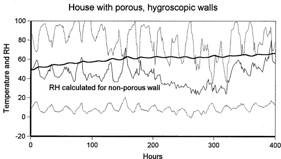
*Figure 5.13 The climate in a wooden hut of the same dimensions as in figure 5.12, with walls 0.1 m thick, porous right through. The air exchange rate is now 0.1 per hour and the room is warmed to a constant 18°C. The wood has the longitudinal direction oriented through the wall, to increase the diffusion rate of water vapour.*
