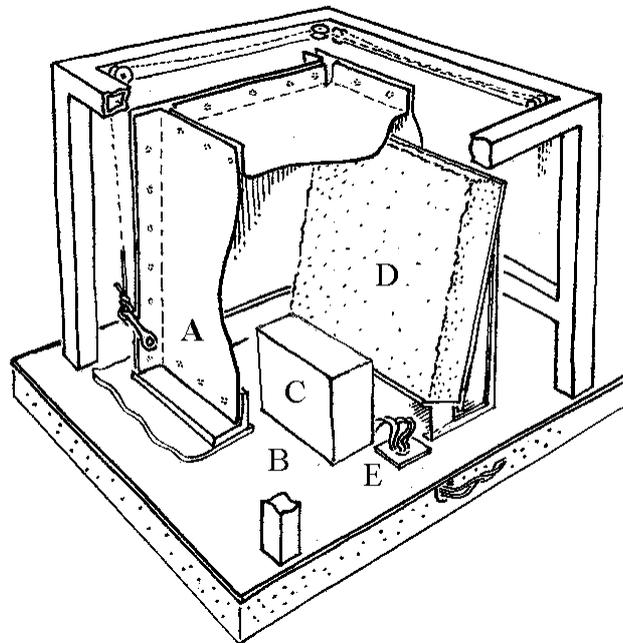
*Figure 2.1 A cut away diagram of the experimental chamber. The scale is distorted to emphasise the main features. It is a stainless steel box **A** without a base, that sits on a stainless steel plate **B**. Electrical and other services **E** are sealed through the base. The experimental wall **D** is tilted back on a support so that it can be constructed of loose blocks. The air conditioning equipment **C** is within the box.*
