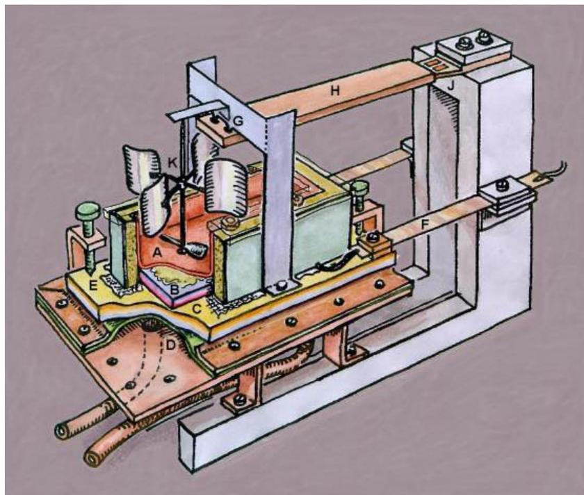
*Figure 2.5 The flux generator. The device is 350 mm long. The cold water tank **A** is made of copper and is clamped down over two thermoelectric coolers **B**. The heat sink for the coolers is the aluminium plate **C**. This is cooled by water circulating in the flat heat exchanger **D**. The top of the heat exchanger is a flexible silicone membrane which is pressed up against the heat sink by water pressure. The vertical displacement of the heat sink is limited by three screws **E**.*
