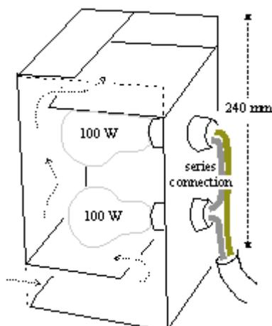
*Figure 2.11 The chamber heater, cut away to show two light bulbs, wired in series to reduce their operating temperature and to increase their lifetime in a regime of constant switching. The case is designed to give good ventilation while allowing little light and radiation to escape.*
