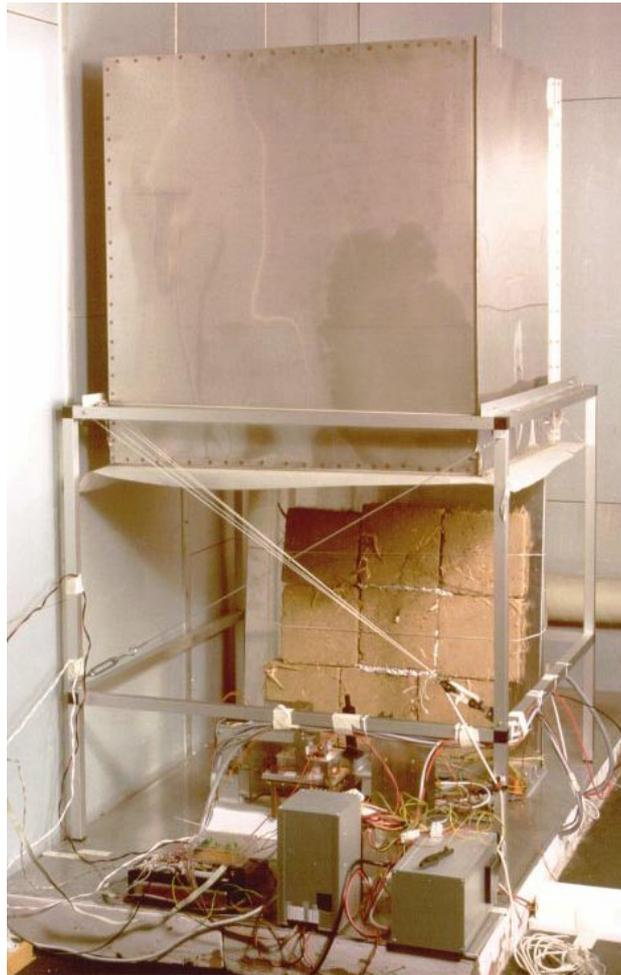
*Figure 2.20 The flux controlling chamber with a wall of stacked mud tiles. The middle tile contains buried sensors. The flux generator and the heater are in the middle distance. In the foreground from left to right: the data logger, the voltage controller for the TEC and the temperature controller. The white object on the right is the insulated water supply to the heat exchanger.*
