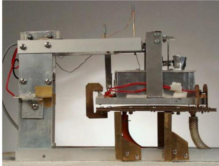
*Figure 2.8 A side view of the apparatus with the cooling water stopped and the membrane collapsed, so that the water tank and heat sink hang free on the weighing beam. Notice the brackets with adjustable screws that restrain the upward movement of the heat sink when the membrane is expanded. These screws are adjusted so that the pins in the stirrup rise just clear of the beam, relieving it of stress and reducing creep. Photo: Christian Bramsen.*
