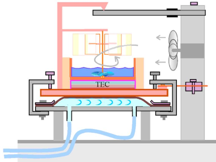
In normal operation the water pressure forces the membrane up against the heat sink of the thermoelectric cooler
