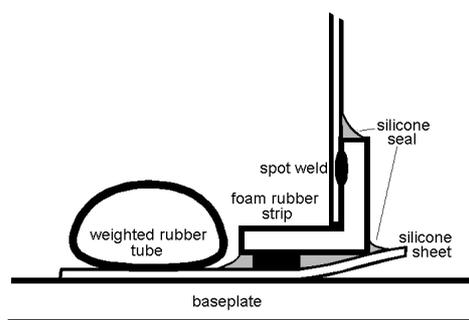
*Figure 2.2 Detail of the seal. The flange around the base of the box has a foam rubber strip stuck underneath it. A wide silicone rubber strip is fixed to the flange with silicone sealant. The foam rubber gives space for the sealant and tilts the silicone so that it tends to press against the base plate. The seal is reinforced by weighted cycle inner tubes laid around the wide skirt which extends over the base plate.*
