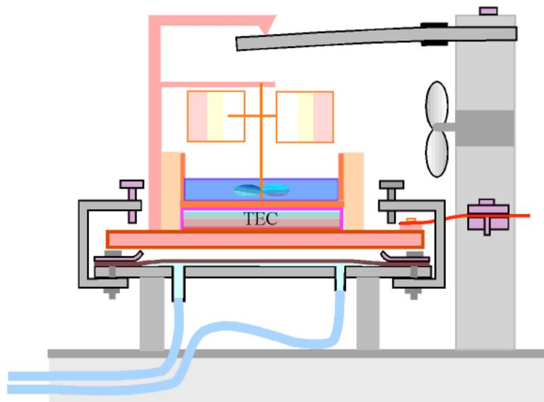
When the water flow stops the membrane collapses and the reservoir hangs from the weighing beam
