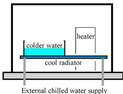
*Figure 2.4 The two temperature principle in flux control: The horizontal radiator controls the air temperature, in competition with the heater. The cooler water tank condenses or evaporates water into the chamber.*
