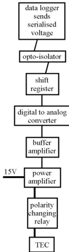
Figure 2.10. Block diagram of the train of instructions from the data logger to the thermoelectric cooler. The TEC takes a high current from a separate power supply, so the data logger control signal is sent first through an optical isolator to guard against electrical interference.
