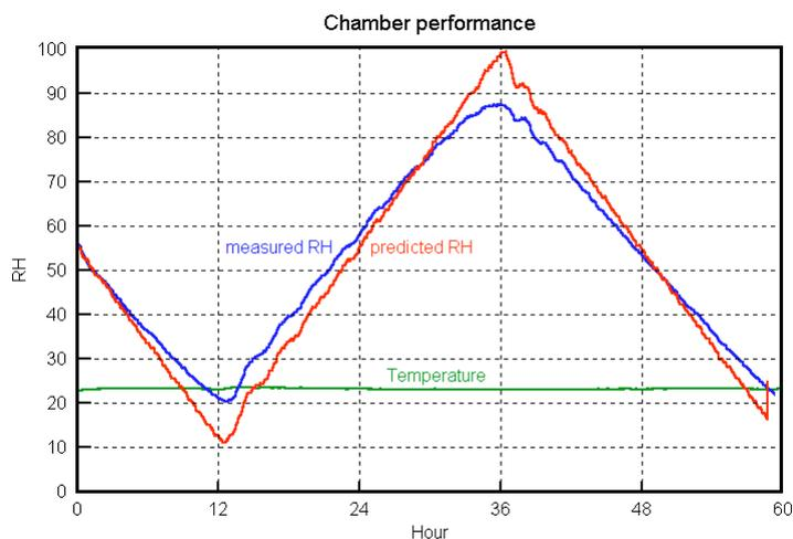
Figure 2.14 The measured RH in the chamber, compared with the RH expected for an inert chamber.
