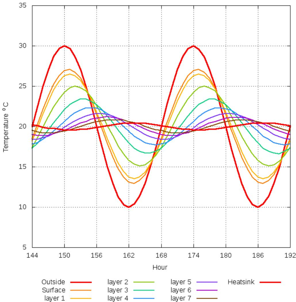
*Temperature distribution through the brick wall. The most wavy trace is the ambient temperature, the flatter central trace (heat sink) is the temperature at the inside surface of the wall. The amplitude of this curve depends on the heat capacity of the room contents.*
