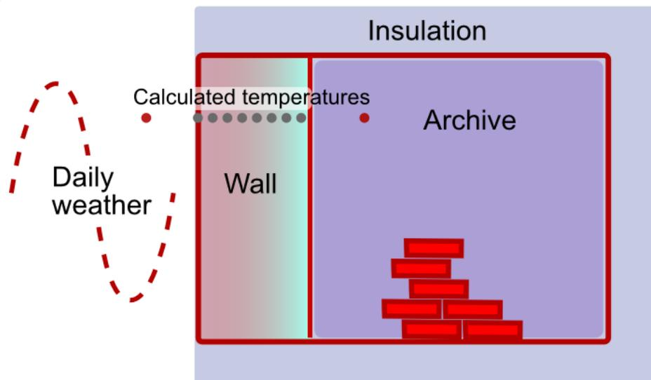
*Model of an archive, characterised by no internal heat source. The heat capacity of the room and its contents is represented by a pile of bricks equivalent to a 200 mm thick brick lining to the room.*
