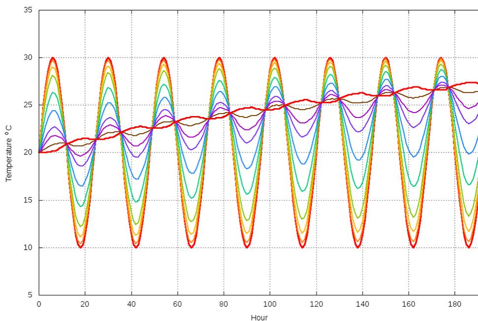
*The temperature in the brick exhibition building (top) rises to an equilibrium about 3 degrees above the average ambient temperature, but the temperature rise in the insulated building is about twice as high.*
