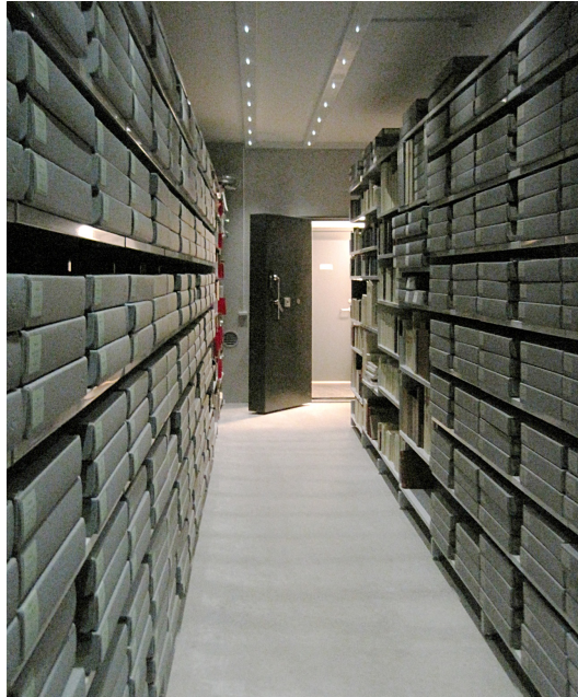
Figure 3: A view of the interior of the archive. It measures 10 \times 4 \times 3 m high. The lobby is visible beyond the armoured and insulated door. The duct for pumped outside air is just visible above and to the left of the door.
