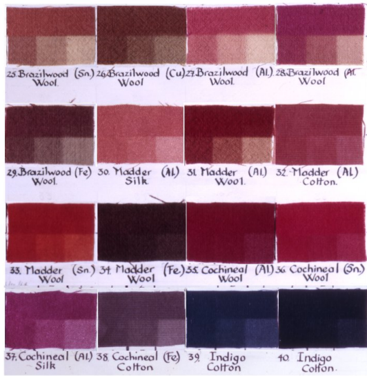
FIG. 1. Some of the faded specimens. The rectangular areas are unexposed. The three square areas on each specimen have been exposed to 7.8, 36 and 91 million lux hours of light from Atlas "Northlight" fluorescent tubes. In all the dyes illustrated here the palest area has received the greatest light dose. The GS difference between exposed and unexposed dye is written on the unexposed part.
