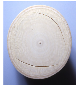
Figure 8: A cross section of an elephant tusk cracked through drying.
