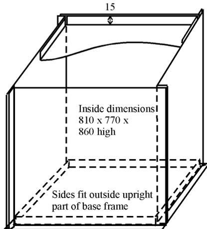
Spot weld just for rigidity: airtightness
