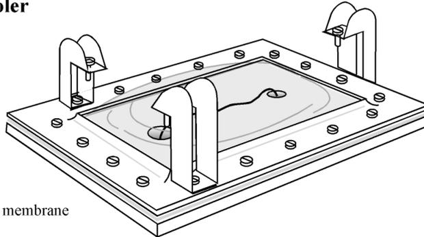
The heat sink is normally forced up against the screws by water pressure under the flexible membrane
