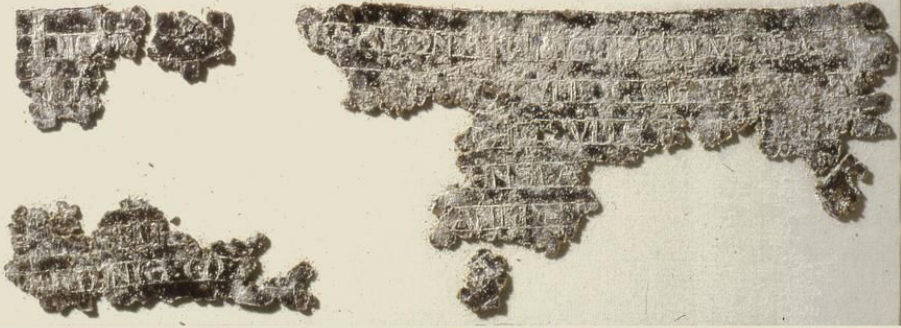
Lead document from an oak coffin, growing white lead carbonate.
