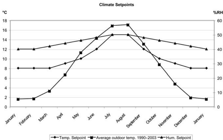
Figure 4. Climate curve with floating set points for temperature and RH approximating the outdoor temperature
