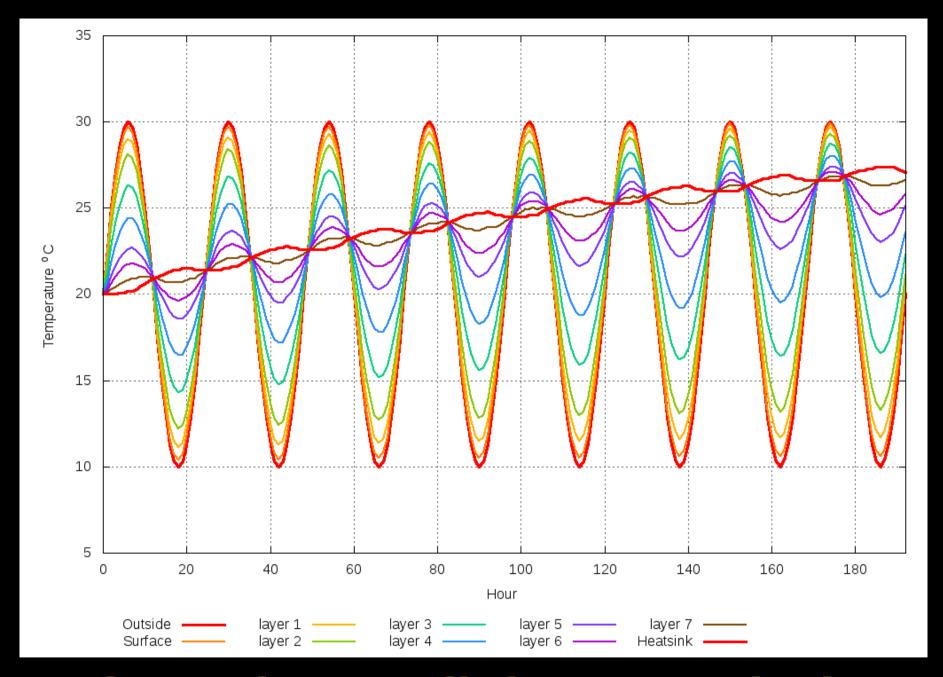
But the insulating wall shows an eight degree temperature rise.
