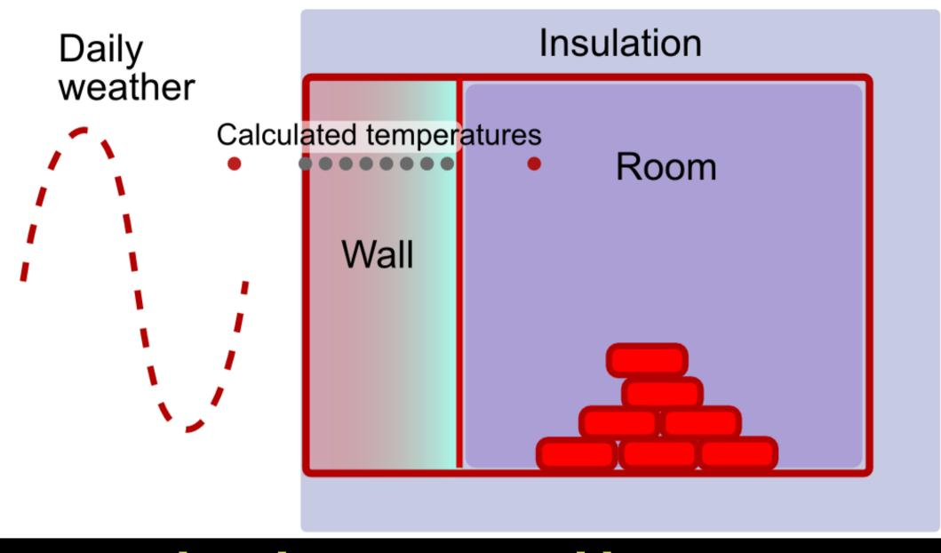
An archive has no internal heat source. The temperature is defined by heat moving through the wall
