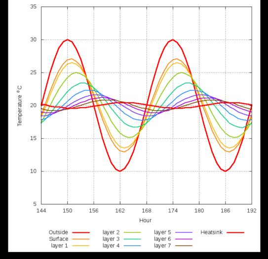
Temperature distribution through a 240 mm brick wall. Heat from the daily outdoor cycle is stored within the wall.
