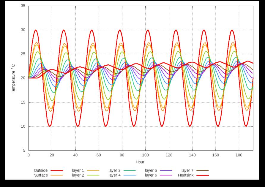
The temperature within the brick museum rises towards a steady state with about four degree temperature rise.
