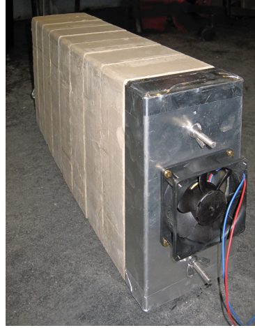
Figure 4: The eight perforated unfired bricks are here assembled with their perforations in line, ventilated by a fan. The outside surfaces were sealed before exposure in the chamber. The wall surface area was 0.1 \text{ m}^2 , the thickness 108 \text{ mm} .
