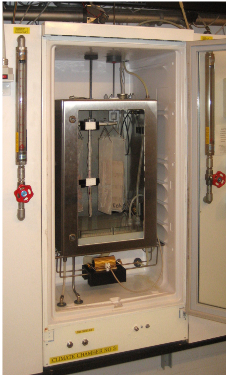
Figure 15: The sorption measuring device. Finely divided specimens are loosely packed in polyester mesh bags which are suspended from a carousel which rotates them in turn to be hooked to a rod, connected via a briefly open tube to a balance mounted out of sight above the picture. The climate is controlled by mixing two air streams, one saturated, the other dry. The entire assembly is held at a constant temperature in a double enclosure.
