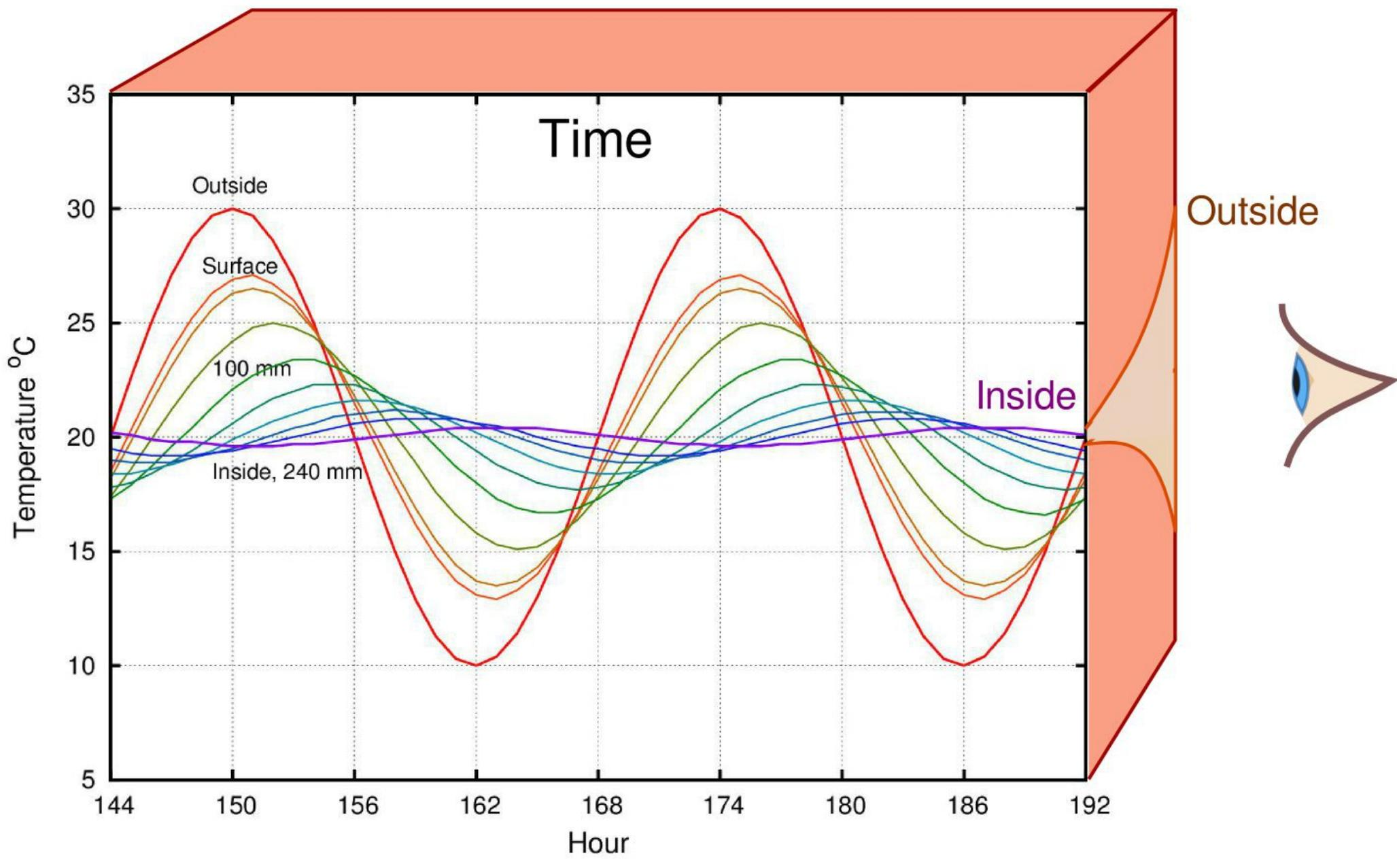
How the daily cycle of temperature penetrates a 240 mm thick solid brick wall
