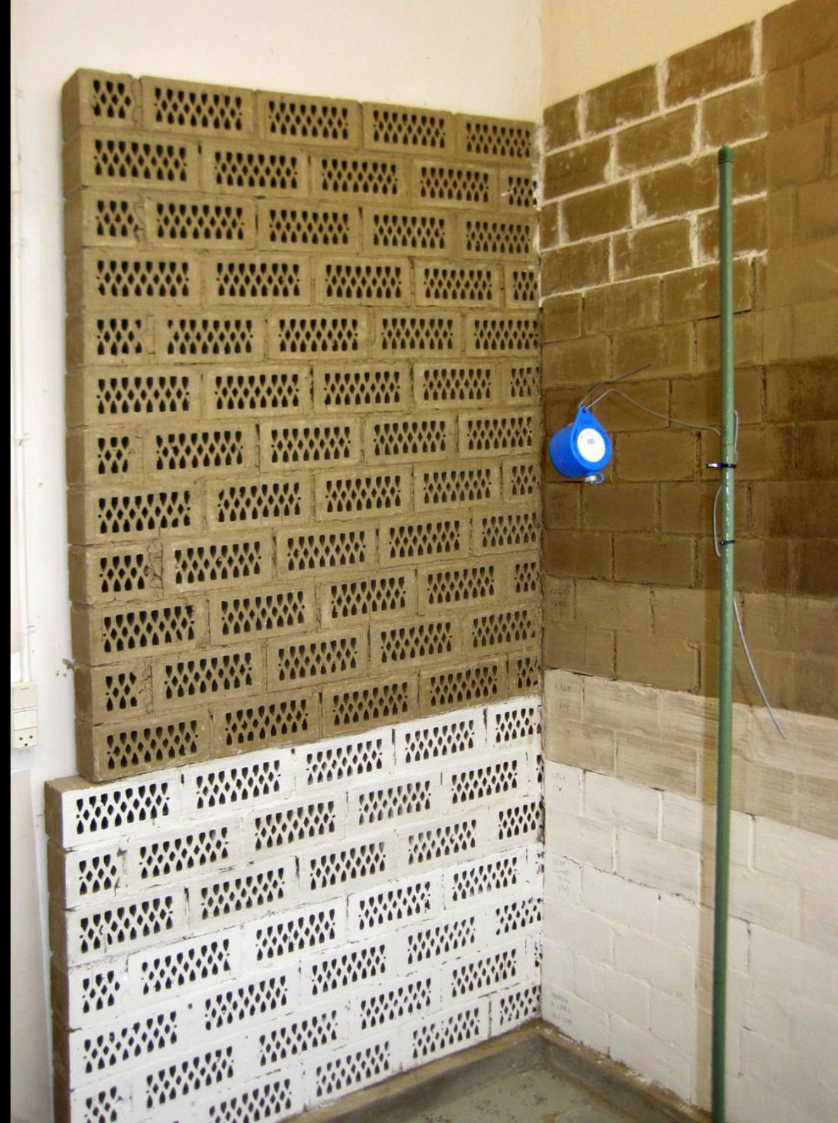
An experimental room partly lined with unfired, perforated clay brick, as a humidity buffer for stores without much absorbent material in the collection
