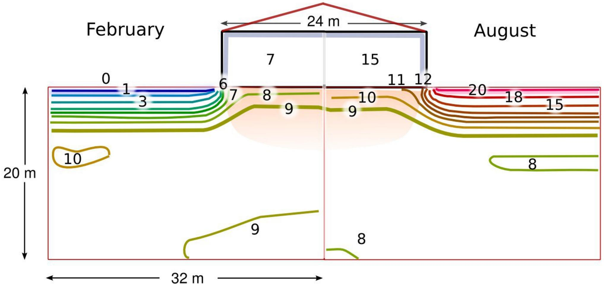
Simulation of the underground temperature contours under a museum store, showing how the ground acts as a huge thermal buffer for the building above
