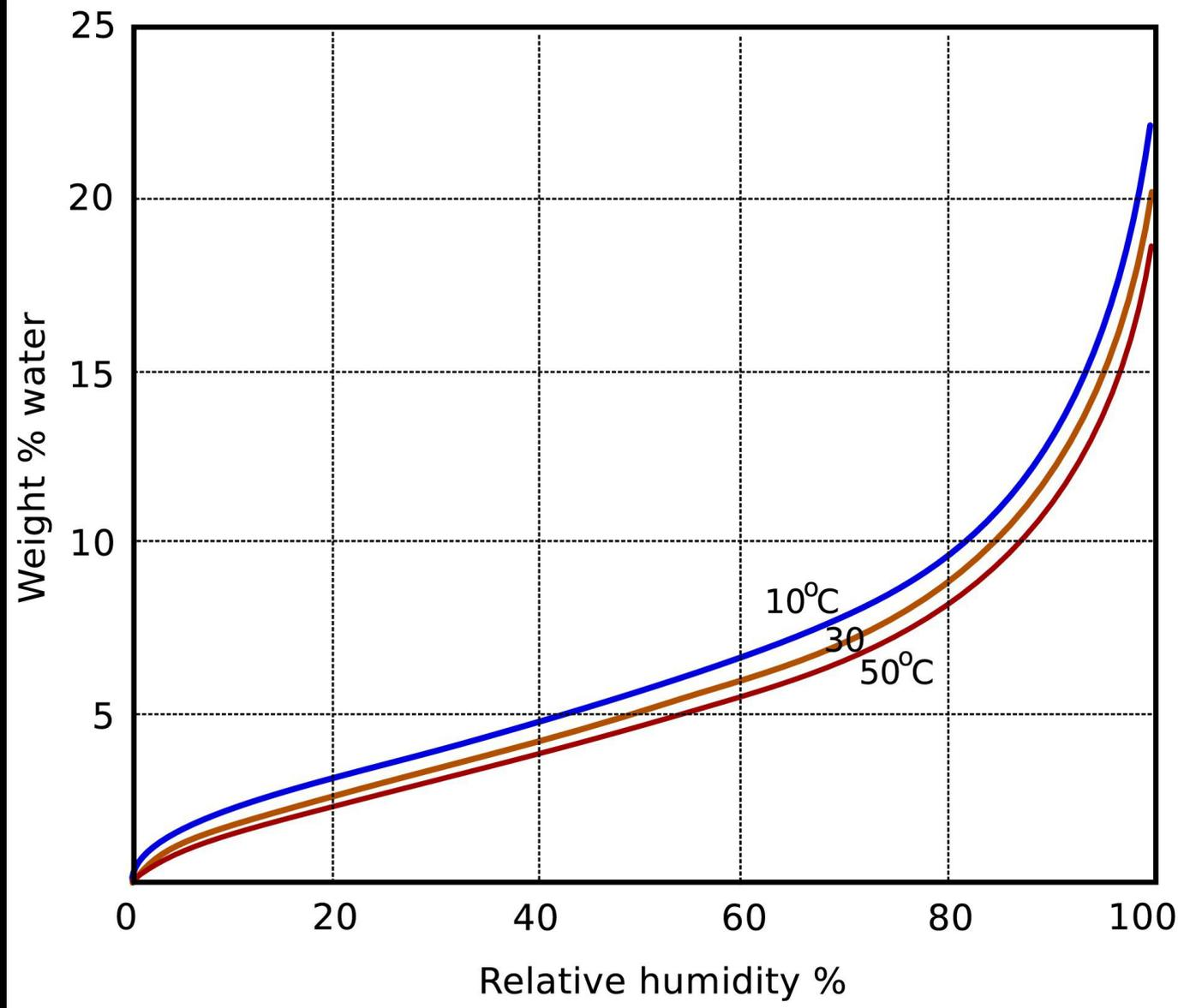
The equilibrium between sorbed water in cotton and water vapour in the space around it is scarcely affected by temperature
