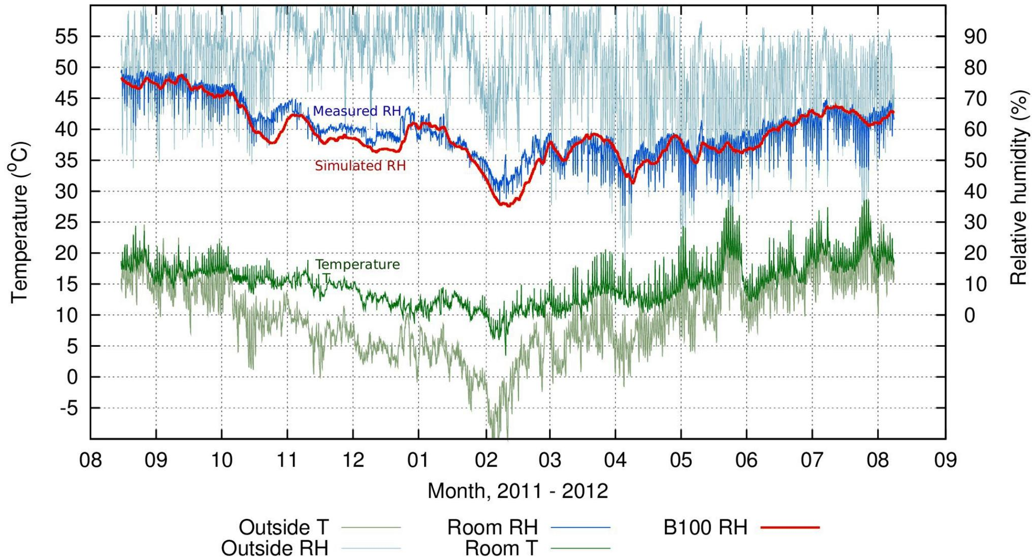
Temperature and RH outside and within the clay lined room. The red trace is the predicted RH. The spikes are due to direct sunlight temporarily overwhelming the buffer capacity of the clay
